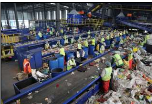
Waste segregation through automated MRFs and its conversion to bales
