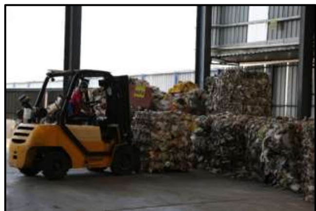
Waste segregation through automated MRFs and its conversion to bales
